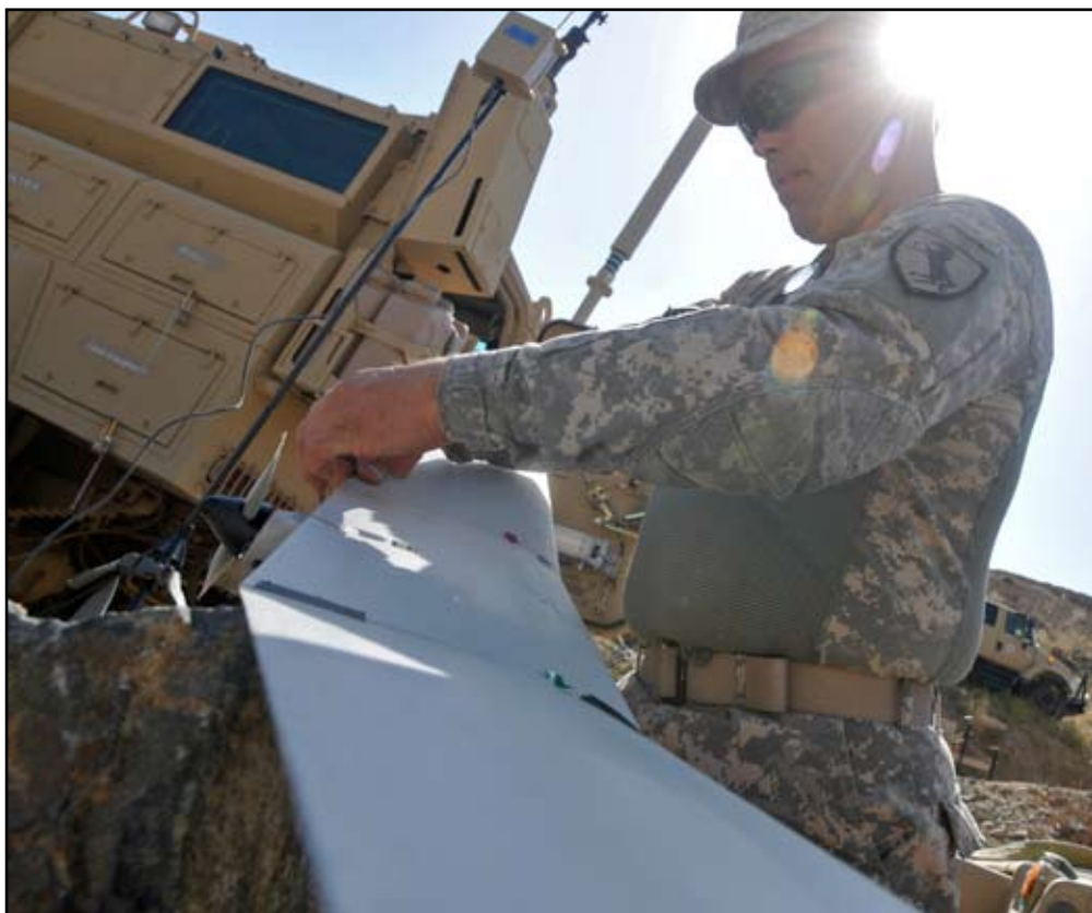
Staff Sgt. Tyrone Baird, master trainer for 1st Squadron, 221st Cavalry Regiment and a Pahrump, Nev., native, assembles the Raven unmanned aerial vehicle at Combat Outpost Nagil, Laghman province, Oct. 13. The Raven is able to provide real time video feeds once in the air.
